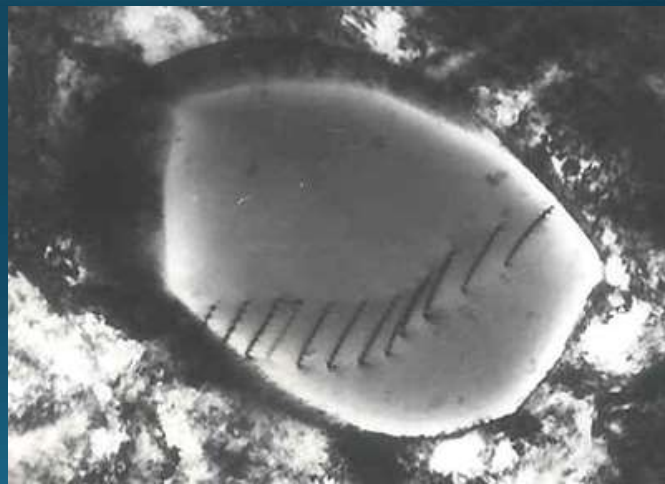
Figure 4.14 Transmitting electron microscope (TEM) image of linear defects, or dislocations. (Photograph courtesy of Andrew Kronenberg.)
