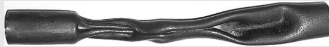
Figure 12.4: A post-strike photograph of a lightning rod fashioned from a hollow copper tube. Figure from Pollock and Barraclough (1905). The authors estimated the current responsible for crushing the tube as \sim 10^5 A. This is the same order of magnitude as lightning-strike currents measured by present-day methods.
