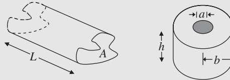
Figure 9.6: A straight wire and a thick washer, both with uniform resistivity \rho = 1/\sigma . Current flows longitudinally through the wire and radially through the washer.
