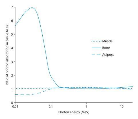
**Figure 6-6.** Energy absorption per X unit (coulomb per kilogram) exposure for several tissues. (Based on data from *Tables of X-Ray Mass Attenuation Coefficients and Mass Energy-Absorption Coefficients from 1 keV to 20 MeV for Elements Z=1 to 92 and 48 Additional Substances of Dosimetric Interest, J. H. Hubbell and S. M. Seltzer, Radiation Physics Division, PML, NIST, 1996. Accessed June, 2016.)*
