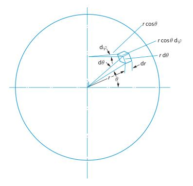
Figure 6-9. Geometry for evaluating Eq. (6.65) for the center of a sphere.
