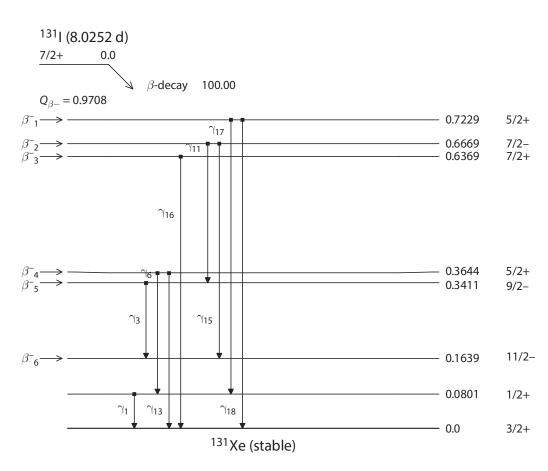
**Figure 6-11.** Transformation scheme for <sup>131</sup>I dosimetry. (Reprinted from: National Nuclear Data Center, Brookhaven National Laboratory, Upton, N.Y., USA.)
