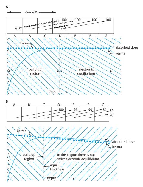
**Figure 6-7. (A)** Graph shows how absorbed dose increases with depth and where electronic equilibrium is achieved when no attenuation of the primary beam occurs; **(B)** attenuation of the beam is included in this figure, and one can see there is no electronic equilibrium past the equilibrium thickness. Units of kerma and dose are the same. (Reproduced with permission from Johns HE, Cunningham JR. *The Physics of Radiology*, 4th ed. Springfield, IL: Charles C. Thomas Publisher, Ltd.; 1983.)
