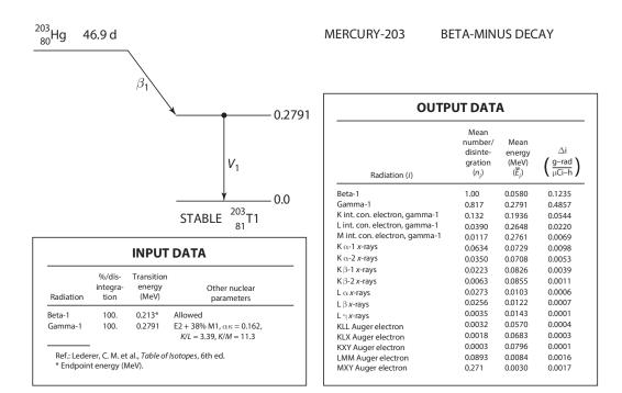
**Figure 6-13.** Transformation scheme and input and output data for <sup>203</sup>Hg dosimetry. (Reprinted by permission of the Society of Nuclear Medicine from Dillman LT. MIRD Pamphlet No. 4: Radionuclide Decay Schemes and Nuclear Parameters for Use in Radiation Dose Estimation. *J Nucl Med.* March 1969; 10(2 Suppl):1–32.)
