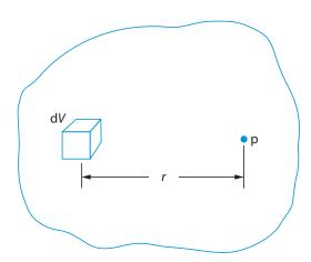
**Figure 6-8.** Diagram for calculating dose at a point p from the gamma rays emitted from the volume element dV in a tissue mass containing a uniformly distributed radioisotope.
