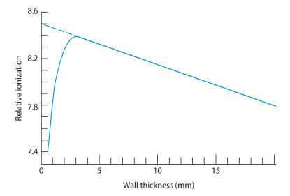
**Figure 6-3.** Ion pairs per unit volume as a function of wall thickness. The ionization chamber in this case was made of pure carbon and was a 20-mm-long cylinder with an inside diameter of 20 mm. (Reproduced with permission from Mayneord WV, and Roberts JE. An attempt at precision measurements of gamma rays. *Br J Radiol*. 1937;10(113):365–386. Permission conveyed through Copyright Clearance Center, Inc.)
