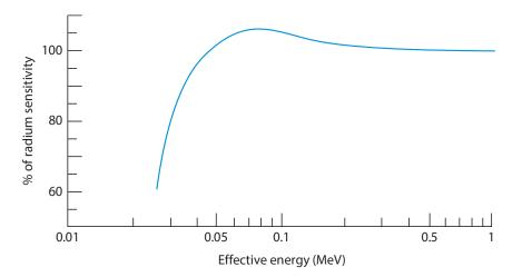
Figure 6-4. Energy dependence characteristics of the pocket dosimeter shown in Figure 9-20.
