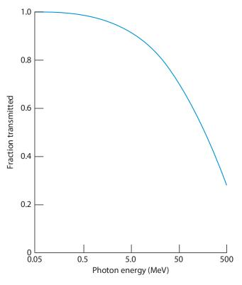
**Figure 6-5.** Fractional number of photons transmitted through an air wall of thickness equal to the maximum range of the primary electrons. (From *Protection Against Betatron—Synchrotron Radiations up to 100 Million Electron Volts.* Washington, DC: US Government Printing Office; 1955. NBS Handbook 55.)
