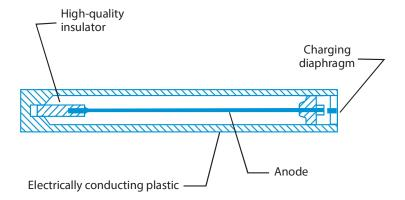
Figure 6-2. Non-self-reading condenser-type ionization chamber.
