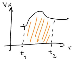
$$\int_{t_1}^{t_2} v_x(t') dt' = \int_{t_1}^{t_2} \frac{dx(t')}{dt'} dt' = \int_{x(t_1)}^{x(t_2)} dx = x(t_2) - x(t_1)$$
