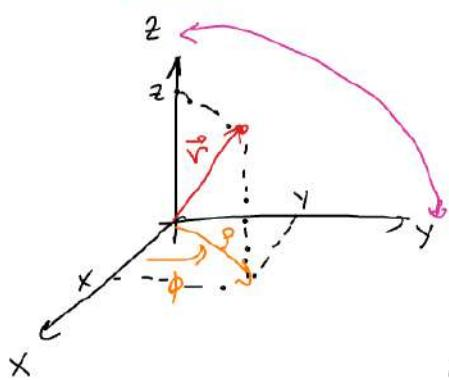
$$\begin{aligned}\vec{r} &= x\hat{i} + y\hat{j} + z\hat{k} \\ x &= p \cos \phi \\ y &= p \sin \phi \\ z &= z\end{aligned}\left.\right\} \quad \boxed{\vec{r} = p \cos \phi \hat{i} + p \sin \phi \hat{j} + z \hat{k}}$$
