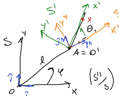
$$\vec{\omega}_{S/S'} = \vec{\omega}_{S'/S} + \vec{\omega}_{S/S'} = \dot{\theta} \hat{k} + \dot{\phi} \hat{k} \\ = (\dot{\theta} + \dot{\phi}) \hat{k}$$
