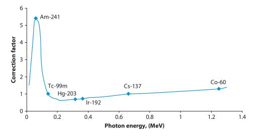
**Figure 13-4.** Energy dependence of a Geiger counter survey meter. The meter reading is multiplied by the correction factor appropriate to the photon energy in order to obtain the true exposure rate. Figure based on data from Ludlum Model 44-9 GM detector.
