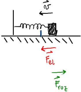
$$m\ddot{x} = \underbrace{-kx}_{-F_{el}} - \underbrace{b\dot{x}}_{+F_{roz}}$$
