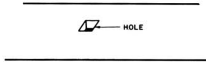
Fig. 7.127. Hole vacancy upon a crystal lattice plane.
