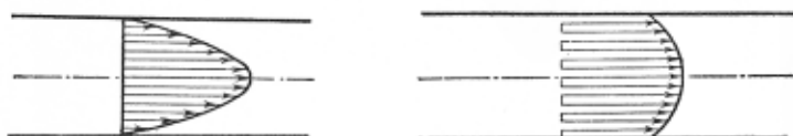
Figure 6. Velocity distribution in laminar (left) and turbulent (right) flow in a tube.
