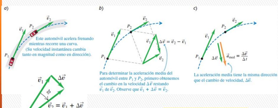
$$\overline{\boldsymbol{a}}_{med} = \frac{\Delta \overline{\boldsymbol{v}}}{\Delta t} = \frac{\overline{\boldsymbol{v}}_2 - \overline{\boldsymbol{v}}_1}{t_2 - t_1}$$
