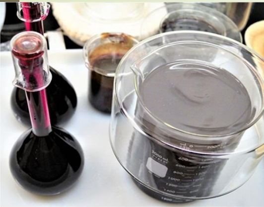
Soaking the glassware for 48 hrs in potassium permanganate solution
