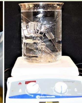
Cleaning glassware with boiling ultra-high purity (UHP) water
