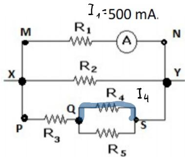
$$R_{eq} = \frac{R_A R_B}{R_A + R_B}$$
