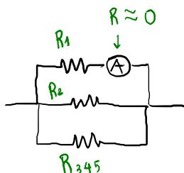
$$R_{12345} = \frac{1}{\frac{1}{R_1} + \frac{1}{R_2} + \frac{1}{R_{345}}} = 0.74 \Omega$$
