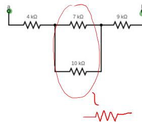
$$R_{eq} = 4.2 \text{ k}\Omega = \frac{1}{\frac{1}{10 \text{ k}\Omega} + \frac{1}{7 \text{ k}\Omega}}$$
