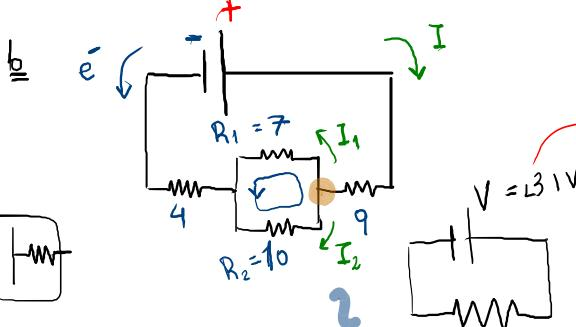
$$\begin{cases} \text{I}_1 R_1 - \text{I}_2 R_2 = 0 & (\text{mallas}) \\ \text{I}_1 + \text{I}_2 = \text{I} & (\text{nodos}) \end{cases}$$
