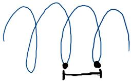
$$v_{\parallel} \cdot \Delta t = \frac{v_{\parallel}}{v_{\perp}} \cdot 2\pi R$$
