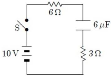
$$R = 9\Omega \quad \left. \begin{array}{l} \\ C = 6\mu F \end{array} \right\} \tau =$$
