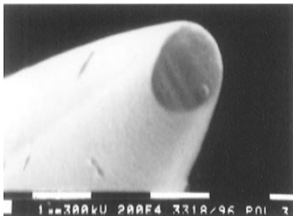
Figure 6.3.3.8 Scanning electron micrographs of 50-nm radius conductive Pt disk somewhat displaced toward the edge of the 1- \mu\text{m} radius glass ring. [Reproduced with permission from Y. Shao, M. V. Mirkin, G. Fish, S. Kokotov, D. Palanker, A. Lewis, Anal. Chem. 69 , 1627 (1997). Copyright 1997, American Chemical Society.]
