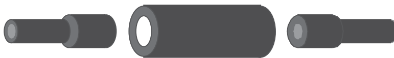
Figure 2.2 Two-electrode cell for solid-state conductivity measurements. (for colour version: see colour section at the end of the book).
