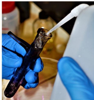
Cleaning the glassware in piranha solution
