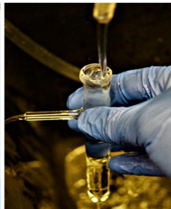
Rinsing glassware with ultra-high purity (UHP) water
