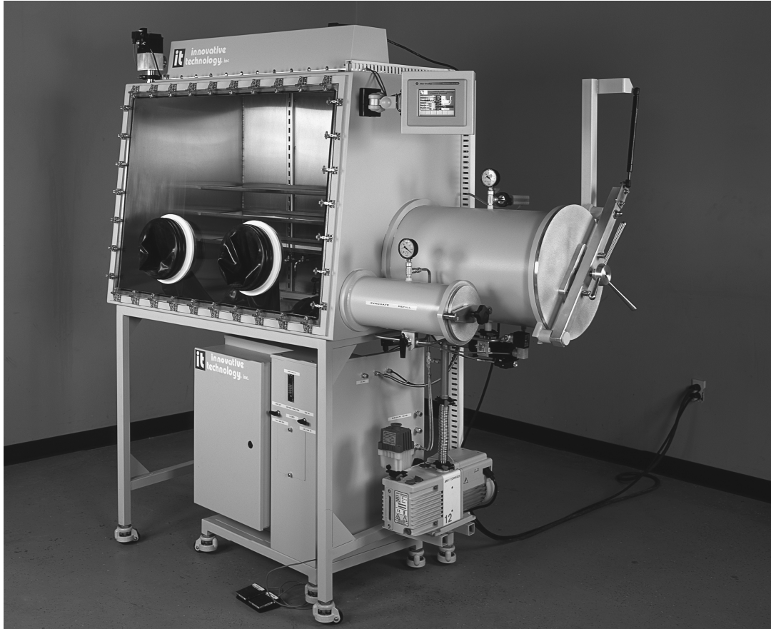
Figure 11-2. Glove box for operations with low-intensity radioactive materials that might accidentally become dispersed into the environment if not handled in an enclosed volume. In use, long rubber gloves fit over the port flanges; material transferred into or out of the glove box through the air lock at the right of the glove box. (Used with permission from Innovative Technology, Inc.)
