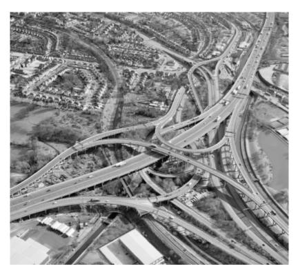
Fig. 14.28 The Gravelly Hill intersection, otherwise known as Spaghetti Junction. This famous, or infamous, interchange is where the M6 (running left to right) meets the separated lanes of the A38(M) (rising from lower right). These major through-routes also join up with local roads, giving access to the nearby city centre. Note also the railway line and the Tame Valley Canal.
