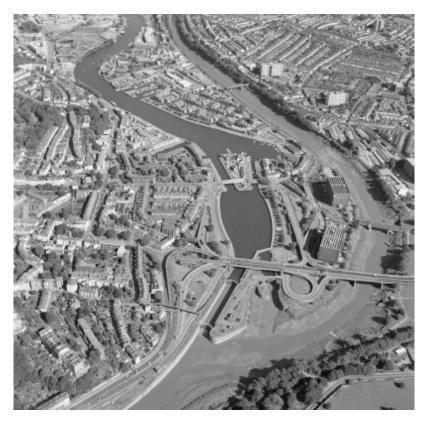
Fig. 13.7 An aerial view of central Bristol looking upstream, with the New Cut (1804–9) to the right (south). The Cumberland Basin is at the centre with its locks. Note the length of the locks, which were designed to hold seagoing vessels. Beyond the Cumberland Basin is the main Floating Harbour, which was entered via the Cumberland Basin. The entire scheme was completed in 1809.
