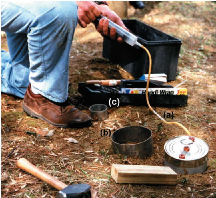
Figure 20.4 Using a soil quality kit in the field. The three different cylinders are for measuring: (a) soil respiration rate, (b) infiltration capacity, and (c) bulk density. (Photo courtesy of Ray R. Weil)
