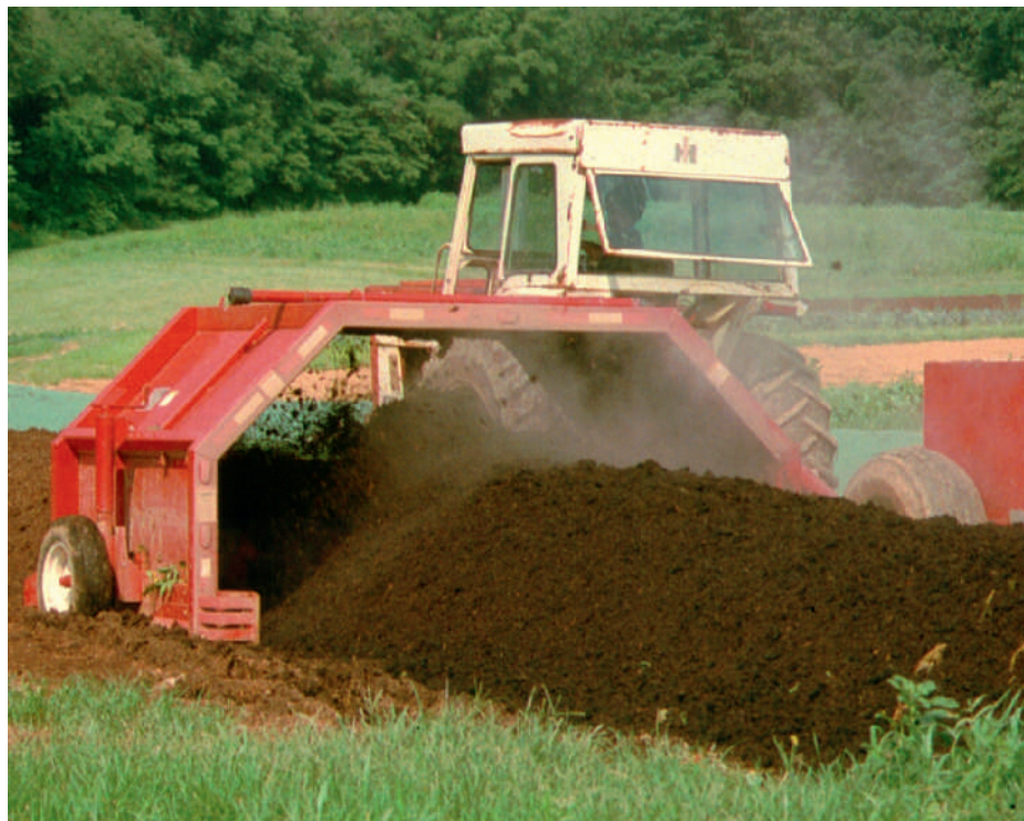
Figure 12.41 A special machine turns large-scale compost windrows (direction of travel is away from the photographer) to mix the material and maintain well-aerated conditions at a facility in North Carolina, USA, where university dining hall food scraps are processed into compost for campus landscaping. (Photo courtesy of Ray R. Weil)
