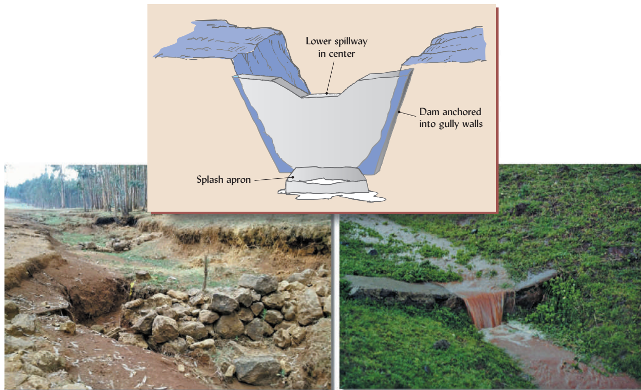
Figure 17.31 A schematic drawing of a check dam used to arrest gully erosion (upper center). Whether made from rock, brush, concrete, or other materials, a check dam should have the general features shown. The structure should be dug into the walls of the gully to prevent water from going around it. The center of the dam should be lower so that water will spill over there and not wash out the soil of the gully walls. An erosion-resistant apron made from densely bundled brush, concrete, large rocks, or similar material should be installed beneath the center of the dam to prevent the overflow from undercutting the structure. An effective check employing these features is shown at the right. In contrast to the gully-healing effect of a well-designed check dam, the haphazard dumping of rocks, brush, or junked cars into a gully will make matters worse, not better (left). (Diagram and photos courtesy of Ray R. Weil)
