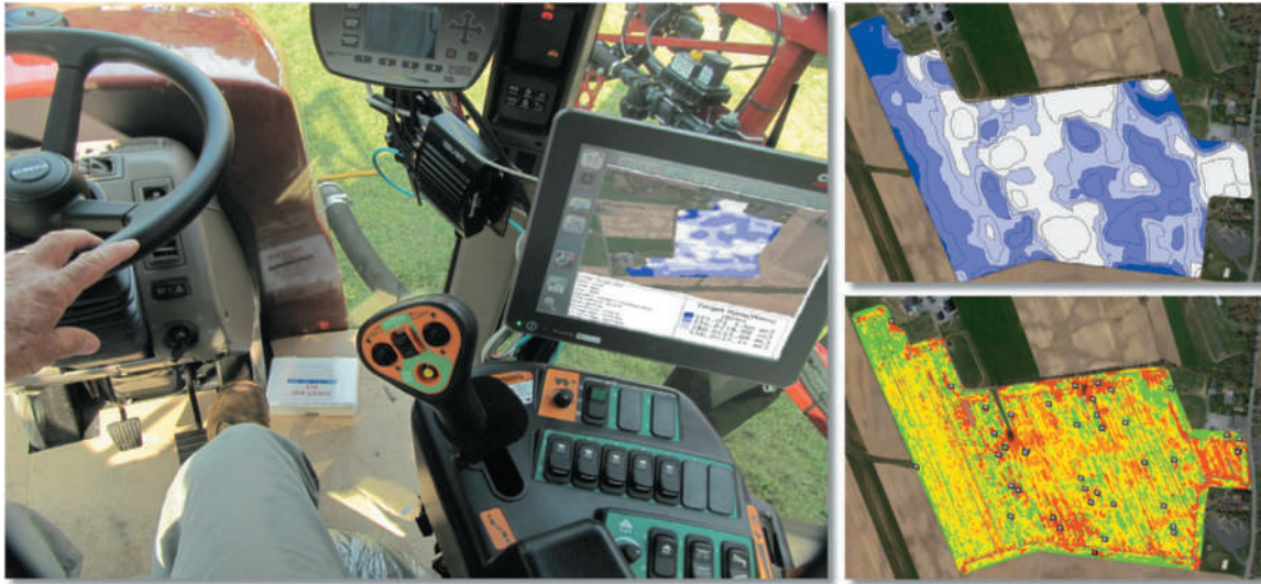
Figure 19.38 Use of GPS technology in precision or site-specific farming. (Left) View from the cab of a fertilizer spreading machine that is GPS-guided and capable of changing the rates of application as required by the computer map as it drives across a field. This type of farming is also known as Prescription Farming. (Upper right) A map of the same field showing the lime required to raise the soil pH to 6.5 as determined from samples collected in 1-ha cells. (Lower right) This map of corn yields throughout a 22-ha field was generated by a harvesting machine equipped with a yield monitor and a GPS receiver. Each dot on the map was generated as the monitor recorded the yield of corn every few meters while the machine worked up and down the field. Each yield measurement was associated with a map position determined by the GPS. An agronomist can then check the red areas where yields were low to ascertain the cause and design measures to alleviate the problem in those spots. (Photo of in-cab computer enhanced to show detail, courtesy of Ray R. Weil, maps courtesy of Hoober, Inc)
