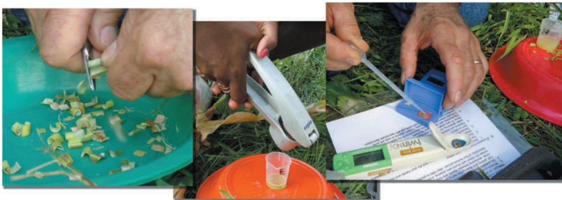
Figure 16.44 Analysis of plant sap in the field. Plant stems or leaf petioles are chopped into small pieces (left) and then squeezed to express a few drops of sap (middle) which is then placed on an ion selective sensor to determine the concentrations of such ions as \text{NO}_3^- or \text{K}^+ . Reference values for sap \text{NO}_3^- and K, as well as tissue analysis norms for those and other elements are given for vegetable crops in Hochmuth et al. (2012). (Photos courtesy of Ray R. Weil)
