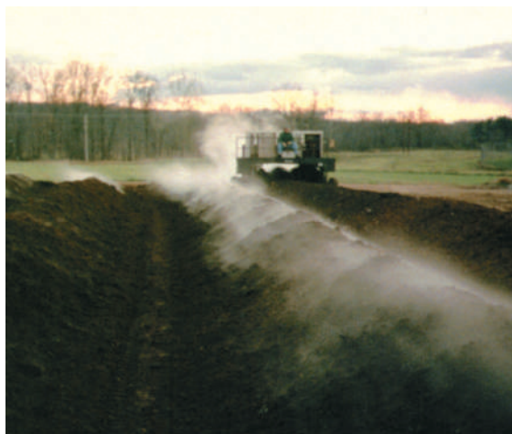
Figure 18.17 Hot water vapor rises in cold winter air as windrows of high-temperature compost are mixed and aerated by a special compost-turning machine in order to accelerate the breakdown of organic compounds. The method can hasten the degradation of organic pollutants in soil material excavated from a contaminated site, mixed with decomposable organic materials, and made into windrows. (Photo courtesy of Ray R. Weil)
