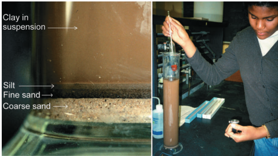
Figure 4.17 In performing particle-size analysis, a sample of soil (with organic matter removed) is suspended in water, stirred vigorously, and then allowed to settle. A hydrometer (right) can indicate the mass of particles remaining in suspension after different settling times (it floats higher when more soil is in suspension). Stokes' Law is used to calculate the smallest effective diameter of the particles still in suspension at these times. (Left) The layers of sand and silt that have settled out after 7 hours. (Photos courtesy of Ray R. Weil)
