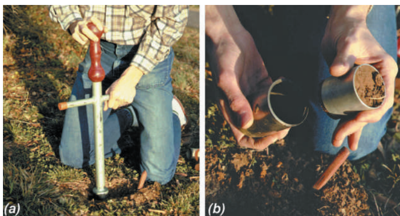
Figure 4.43 A special sampler designed to remove a cylindrical core of soil without causing disturbance or compaction (a). The sampler head contains an inner cylinder and is driven into the soil with blows from a drop hammer. The inner cylinder (b) containing an undisturbed soil core is then removed and trimmed on the end with a knife to yield a core whose volume can easily be calculated from its length and diameter. The weight of this soil core is then determined after drying in an oven. (Photos courtesy of Ray R. Weil)
