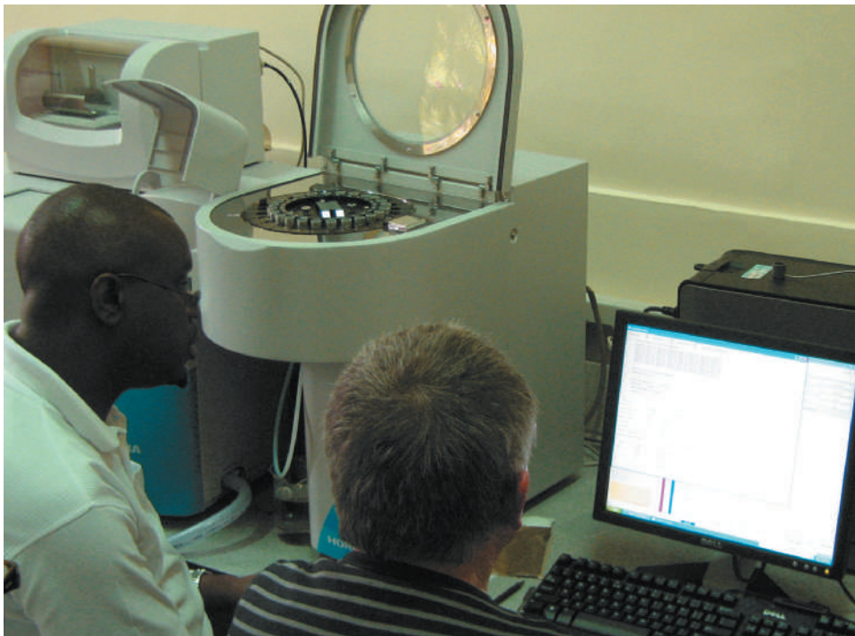
Figure 4.18 A computerized and semi-automated laser diffraction instrument is used to analyze soil particle size distribution in a lab in Kenya. Laser light is diffracted ("bent") at greater angles by smaller particles. Therefore, when parallel laser light beams pass through a dispersed soil sample suspended in water, the intensity of the diffracted light sensed at different angles from the sample can be interpreted through a set of complex calculations to indicate the number of particles of any particular diameter. For a comparison of strengths and weaknesses of laser and sedimentation methods see Di Stefano et al. (2010) (Photo courtesy of Ray R. Weil)
