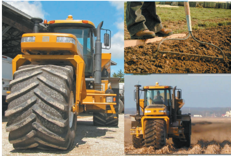
Figure 4.52 One approach to reducing soil compaction is to spread the applied weight over a larger area of the soil surface. Examples are extra-wide wheels on heavy vehicles used to apply soil amendments (right) and standing on a wooden board while preparing a garden seedbed in early spring (inset). (Photos courtesy of Ray R. Weil)
