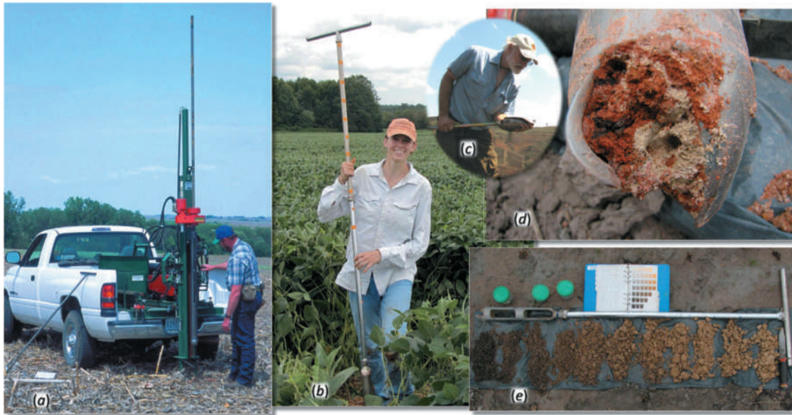
Figure 19.7 Soil maps are prepared by soil scientists who examine the soils in the field using such tools as a truck-mounted hydraulic soil probe (a) or a hand-powered soil bucket auger (b). About a 10-cm depth increment of soil is typically retrieved with just two or three revolutions of the typical bucket auger. After pulling the auger from the ground, but before emptying its load of soil, it is advisable to carefully examine the soil exposed at the end of the auger bucket to observe the relatively undisturbed colors and structure of the soil (c,d). Soil scientists may lay each soil increment in order on a sheet of plastic or in a trough to examine later (e). This allows the colors and textures to be efficiently determined while also presenting an overall view of the soil profile. (Photo (a) courtesy of USDA/NRCS, other photos courtesy of Ray R. Weil)
