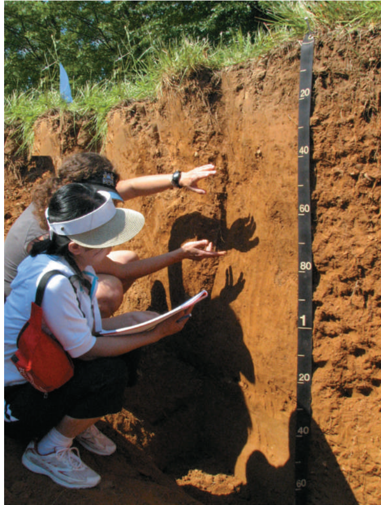
Figure 19.6 A soil pit allows detailed observations to be made of the soil in place. Here, two soil scientists describe a typical pedon for a mapping unit (Pamunkey soil series) as revealed on the wall of a soil pit. The soil scientists are comparing the colors and textures of soil samples removed from several horizons and recording the observations in a notebook to make a soil profile description (such as the one in Table 19.1). Later, when the soil scientists are boring transects of auger holes to map soils in a landscape (see Figures 19.7 and 19.8), they can determine the identity of the soils they encounter by comparing the properties of samples brought up in their augers to the properties listed in detailed written descriptions of the soil pit. (Photo courtesy of Ray R. Weil)
