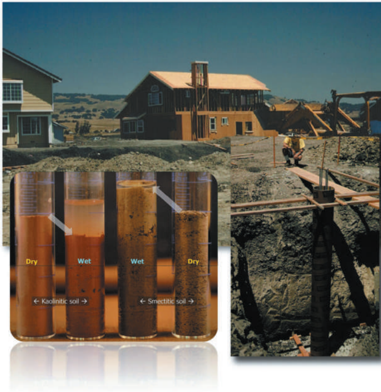
Figure 4.62 The different swelling tendencies of two types of clay are illustrated in the lower left. All four cylinders initially contained dry, sieved clayey B horizon soil, the two on the left are a kaolinitic soil, the two on the right are smectitic. An equal amount of water was added to the two center cylinders. The kaolinitic soil settled a bit and was not able to absorb much of the water. The smectitic soil swelled about 25% in volume and absorbed nearly all the added water. The scenes to the right and above show a practical application of knowledge about these clay properties. Soils containing large quantities of smectite undergo pronounced volume changes as the clay swells and shrinks with wetting and drying. Such soils (e.g., the California vertisol shown here) make very poor building sites. The normal-appearing homes (upper) are actually built on deep, reinforced-concrete pilings (lower right) that rest on nonexpansive substrata. The 15–25 such pilings needed for each home more than doubles the cost of construction. (Photos courtesy of Ray R. Weil)
