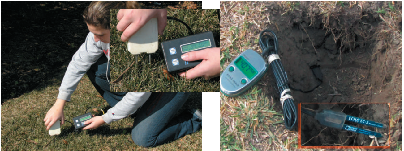
Figure 5.16 Electronic instruments can measure volumetric water content of soil by determining dielectric (insulating) properties of the soil into which a sensor is inserted. A time domain reflectometry (TDR) meter, and sensor (left) and a capacitance sensor and meter (right) are shown. The TDR instrument calculates the volumetric water content of soil by analyzing the velocity at which electromagnetic waves move through the soil and the reflected wave patterns generated. Electrical capacitance probes determine volumetric water content by measuring the amount of charge required to raise the voltage between two conductors separated by the soil. The capacitance instruments are simpler and less expensive than the TDR instruments, but are more likely to require laborious soil-specific calibration. For both methods it is important that the sensors be installed such that the prongs are completely and snugly buried in soil with no air gap. (Photos courtesy of Ray R. Weil)
