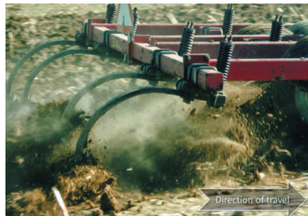
Figure 17.49 A chisel plow in action. Tillage implements such as this loosen and move large quantities of soil, some of which is thrown into the air. The amount of a certain soil that will be moved and the distance it is moved depend on the design of the implement, depth of tillage, and speed of travel. The soil moves mainly in the direction of travel, but will move much farther when travel is downslope so gravity assists the movement. When tillage is upslope, gravity hinders the forward movement of soil. (Photo courtesy of Ray R. Weil)
