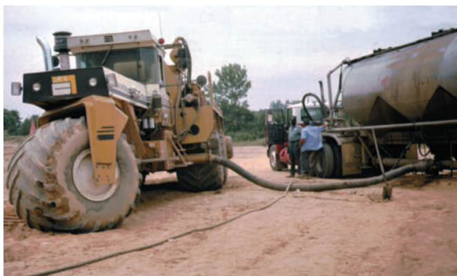
Figure 18.29 Sewage sludge slurry being transferred from a tanker truck to a floatation tire spreader for injection into soils during an ecological restoration project on orphan mined land. Such sludge applications are closely regulated on the basis of allowable metal levels in soil and sludge.
