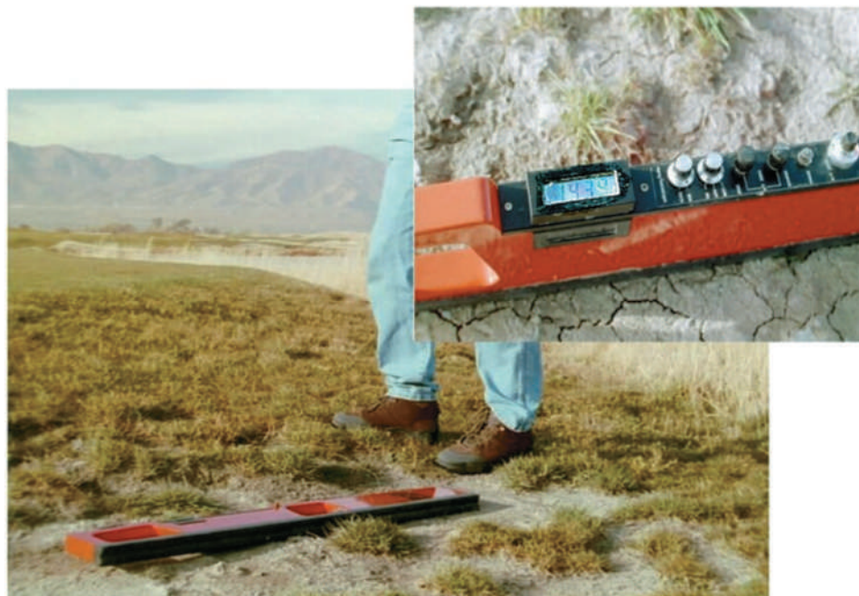
Figure 10.20 A portable electromagnetic (EM) soil conductivity sensor used to estimate the electrical conductivity in the soil profile. When placed on the soil surface in the horizontal position (lower left), this instrument senses electrical conductivity of the soil down to about 1 m depth. When placed in the vertical position (as in the inset photo), the effective depth is about 2 m. (Photos courtesy of Ray R. Weil)
