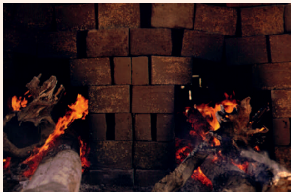
Figure 8.8 In highly weathered regions of the world, people dig up kaolinitic clay soil, mix it with water, mold it into blocks, dry the block in the sun, and then stack them to form a kiln by which they are fired to make bricks. (Photo courtesy of Ray R. Weil)
