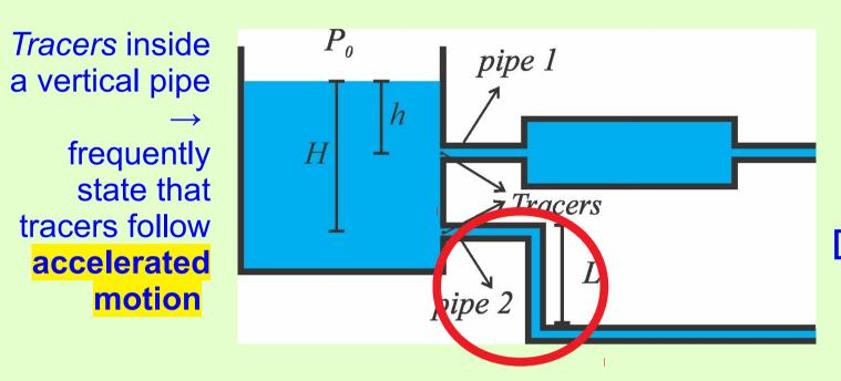
Fluid portions as freefalling particles Non-interacting elements.
