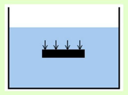
Force on a fluid element is exerted only by the fluid above it
