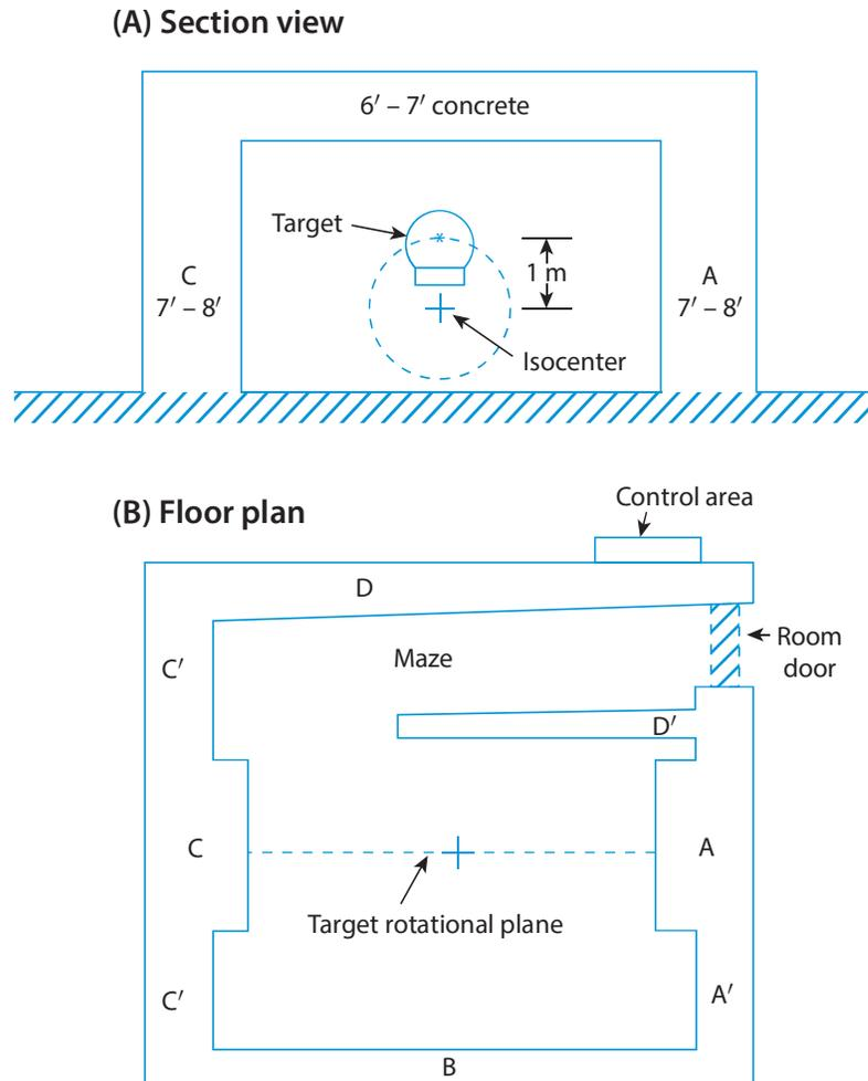
**Figure 10-20.** Simplified schematic of a typical high-energy treatment room. All barriers are constructed of standard concrete ( $147 \text{ lb ft}^{-3}$ ). (Reproduced with permission from McGinley PH. *Shielding Techniques for Radiation Oncology Facilities*. 2nd ed. Madison, WI: Medical Physics Publishing Corp; 2002: Fig 2-1, p. 10.)
