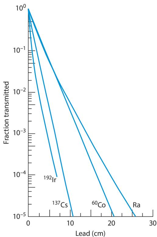
**Figure 10-8.** Broad-beam attenuation by lead of gamma-rays from  $^{192}\text{Ir}$ ,  $^{137}\text{Cs}$ ,  $^{60}\text{Co}$ , and radium. (Reproduced from *Protection Against Radiations from Sealed Gamma Sources*. Washington, DC: National Bureau of Standards; 1960. NBS Handbook 73.)
