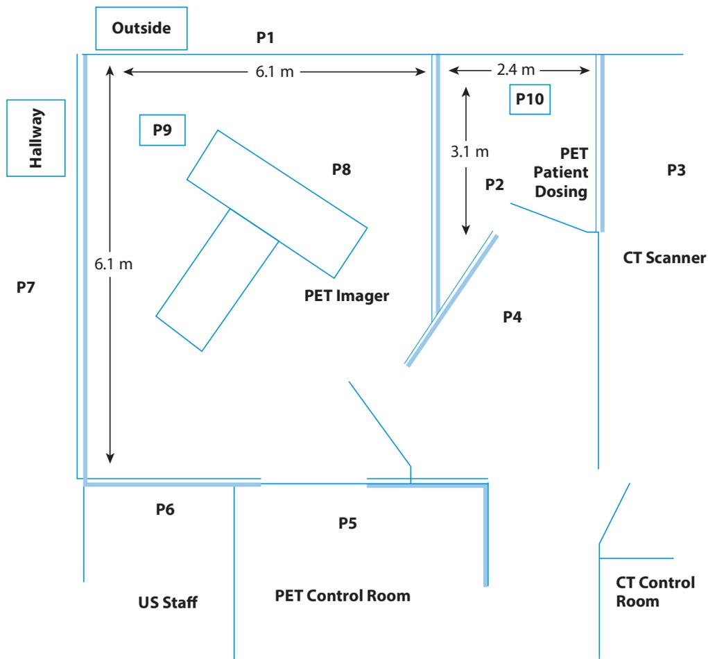
**Figure 10-19.** Plan view of PET suite showing physical dimensions of the imaging room and the patient dosing room. Also indicated are the dose points, P, of interest. Not drawn to scale. (Reproduced with permission from Methé BM. Shielding design for a PET imaging suite: a case study. *Health Phys.* 2003;84(5 Suppl):S83–S88.)
