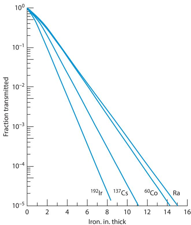
**Figure 10-7.** Broad-beam attenuation by iron of gamma-rays from  $^{192}\text{Ir}$ ,  $^{137}\text{Cs}$ ,  $^{60}\text{Co}$ , and radium. (Reproduced from *Radiological Health Handbook*. Rev ed. Washington, DC: U.S. Government Printing Office; 1970.)
