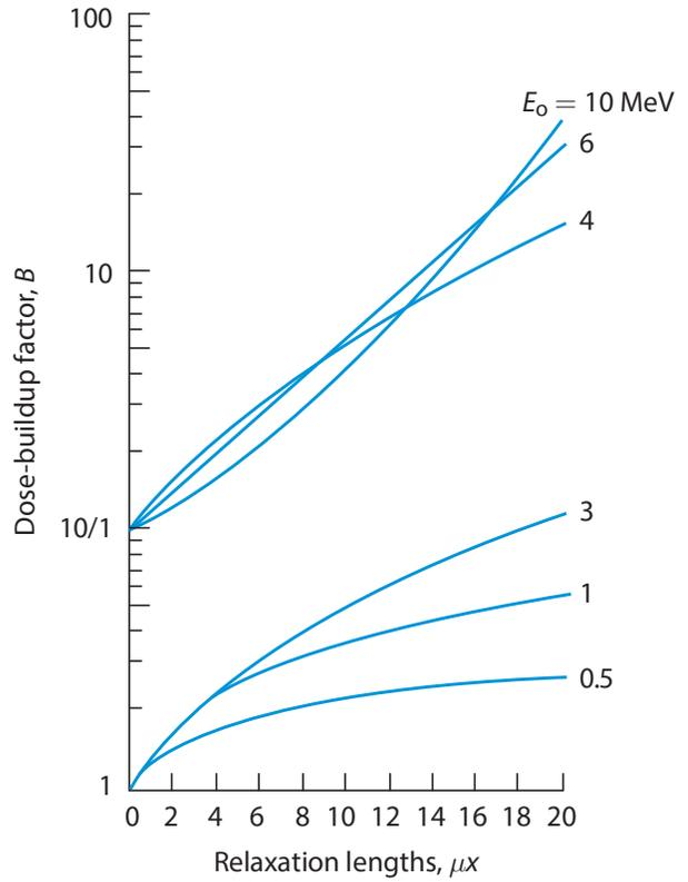
**Figure 10-10.** Dose-buildup factor in lead for a plane monidirectional gamma-ray source of quantum energy  $E_0$ . The 10 in 10/1 on the ordinate applies to the lower curves, while the 1 in 10/1 on the ordinate applies to the upper curves. (Reproduced from *Radiological Health Handbook*. Rev ed. Washington, DC: U.S. Government Printing Office; 1970.)
