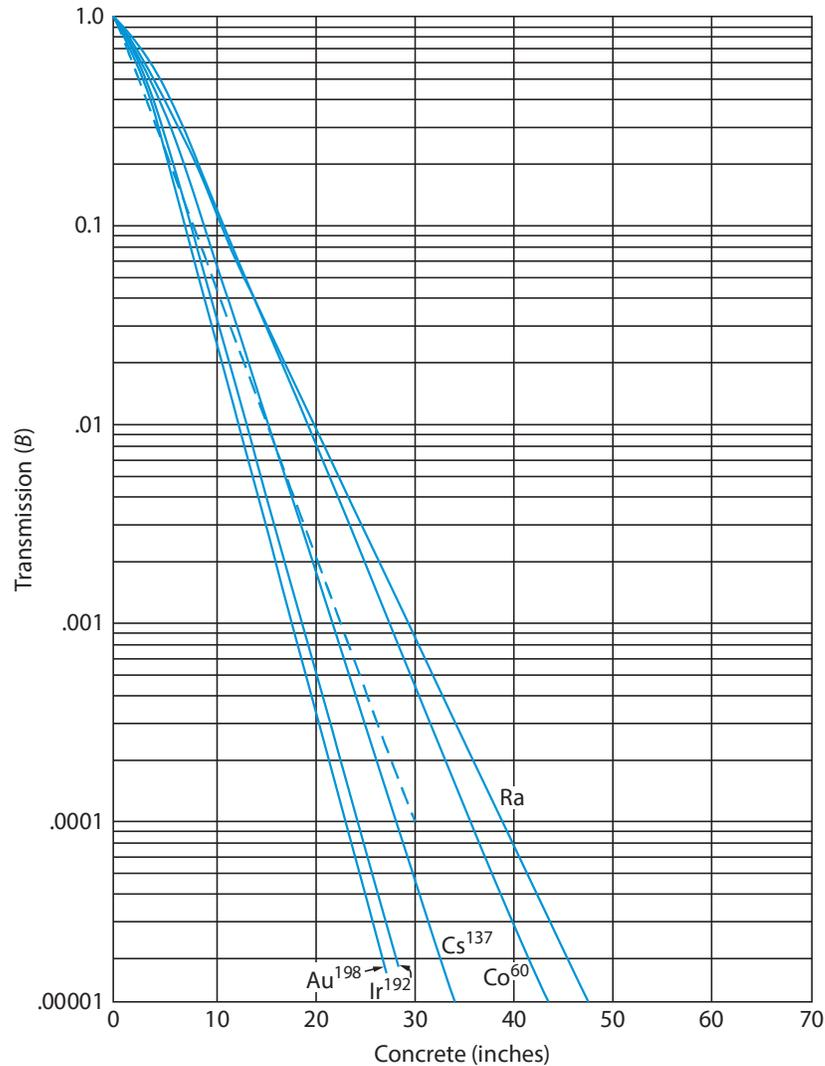
**Figure 10-6.** Fractional transmission of gamma rays from  $^{137}\text{Cs}$ ,  $^{60}\text{Co}$ , and Ra (in equilibrium with its decay products) through concrete. The solid curves represent transmission of broad beams, and the broken line represents  $^{60}\text{Co}$  gamma-ray attenuation under conditions of good geometry. (Reproduced from *Radiological Health Handbook*. Rev ed. Washington, DC: U.S. Government Printing Office; 1970.)
