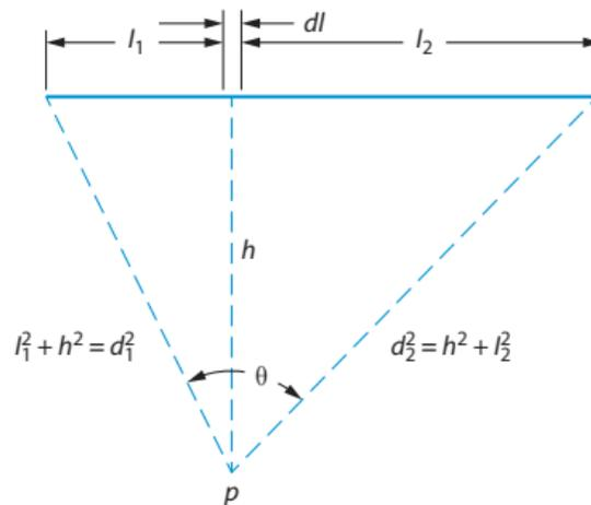
**Figure 10-1.** Geometry for computing gamma-ray dose rate at a finite distance  $h$  from a line source of uniform activity  $C_1$  per unit length.
