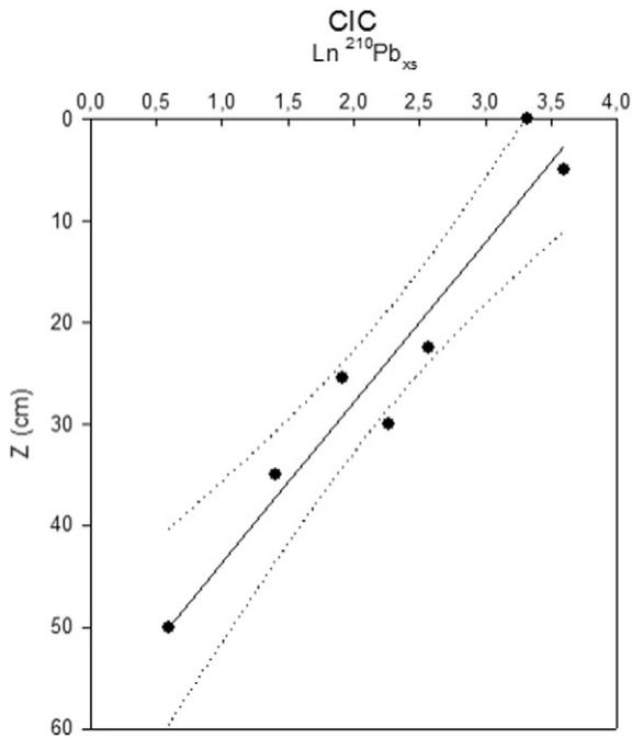
Fig. 2. Plot of  $\text{Ln}^{210}\text{Pb}_{\text{xs}}$  activity vs. depth for BAT1 core. Solid line represents the regression line and dotted lines define the 95% confidence band.
