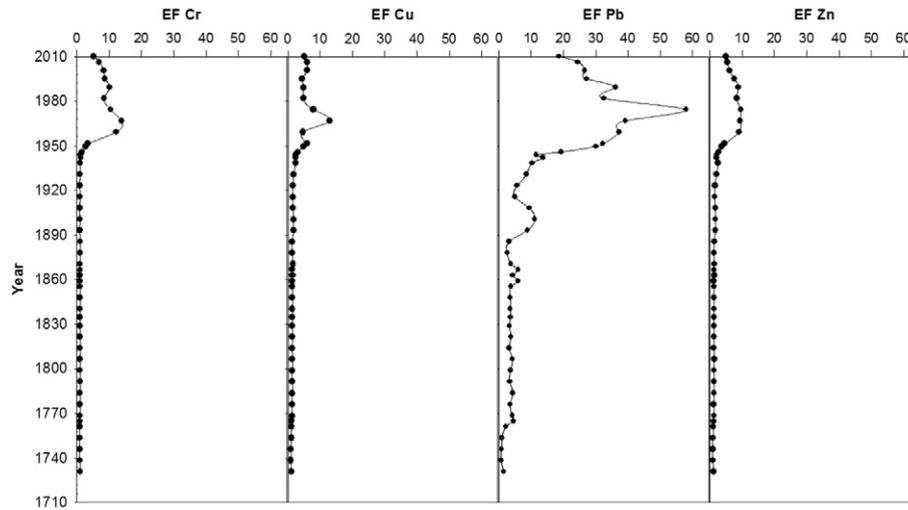
Fig. 4. Enrichment Factor (EF) for Cr, Cu, Pb and Zn.
