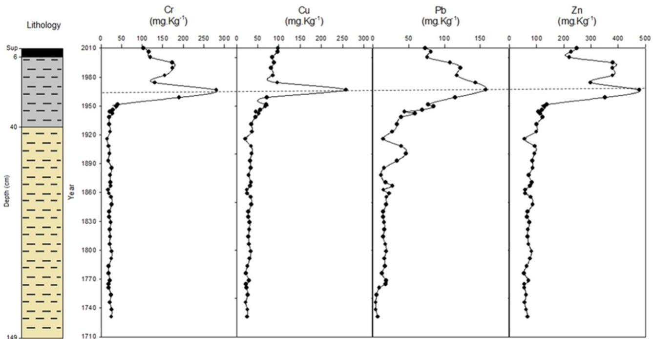
Fig. 3. Lithology and concentrations of Cr, Cu, Pb y Zn ( $\text{mg} \cdot \text{kg}^{-1}$ ) in sediment core BAT1. With a dotted line highlighting the 24th stratum, where the maximum metal concentrations are observed.
