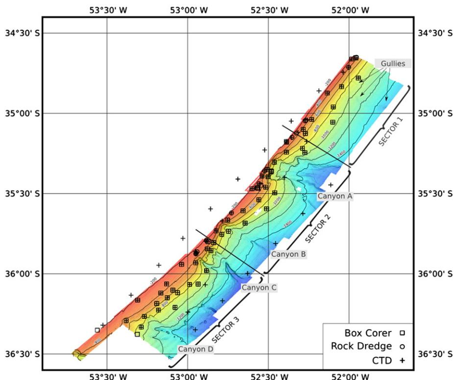
**Fig. 2.** Multibeam coverage of the study area (see Fig. 1 for regional location) showing canyons and gullies, the delimited latitudinal sectors (sectors 1, 2 and 3) and sedimentological and hydrological sampling stations.
